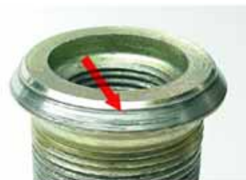
Unevenness of inner nut seating surface (exmaple of iron inner nut)
