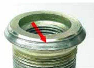
Unevenness of inner nut seating surface (exmaple of iron inner nut)
