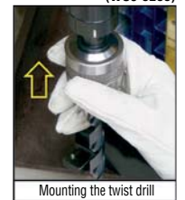
Mounting the twist drill
